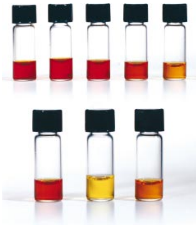
Figure 3. Homogeneous and transparent solutions of NT/PPA (sample from Table 1, no. 1) in THF with concentrations ( c ) of (upper panel from left) 19.07, 10.59, 7.15, 5.45, and 3.18 mg/mL. For comparison, THF solutions of NT/PPA and PPA with similar concentrations are given in the lower panel with c (mg/mL; from left) of 5.45 (NT/PPA), 4.00 (PPA), and 3.18 (NT/PPA).
